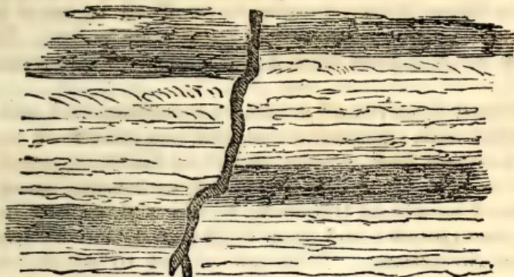
bed above the lowermost strata. In other words, if the dike makes an acute angle with the upper surface of the coal-vein, the strata are elevated on that side; while, if the angle is obtuse, they are thrown down.
